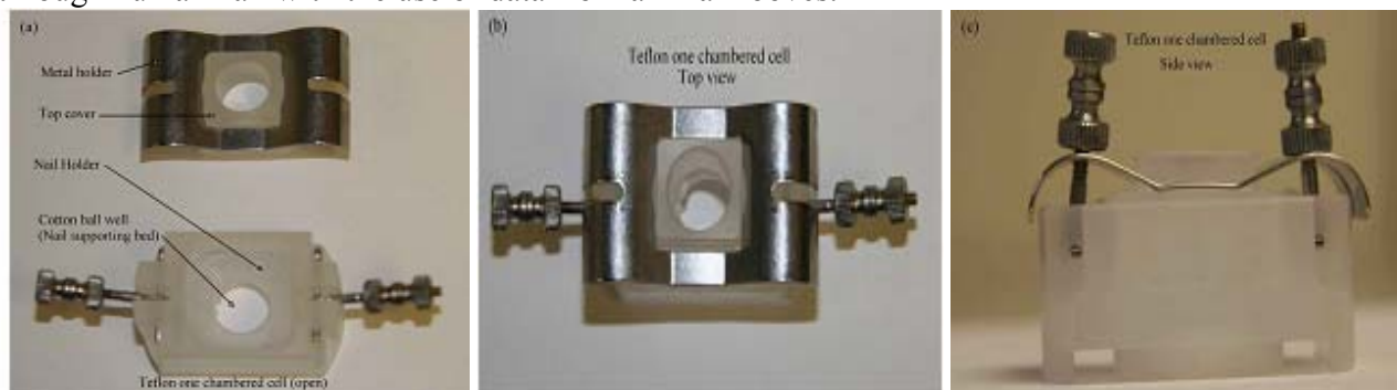
Fig. 5: Nail support and incubation system: (a) Teflon one chamber diffusion cell components, (b) Teflon one-chamber diffusion cell top view, and (c) Teflon one chamber diffusion cell side view.
