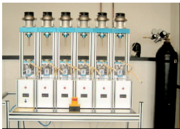
Chewing machines at Pharmalytics used for testing medicated chewing gum.
