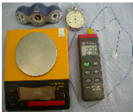
Fig.1: Experimental setup for measuring the temperatures of the exothermic reaction of polymerization of materials for provisional restorations.
