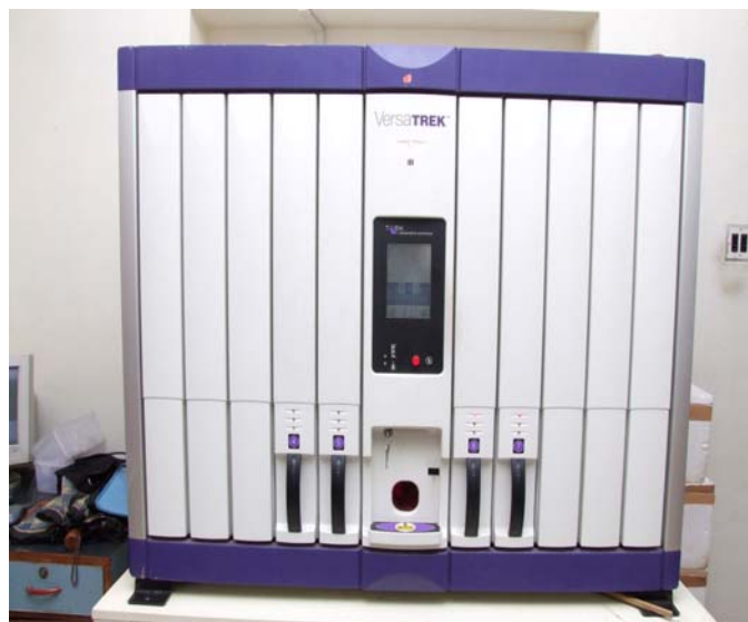
Versa TREK Rapid culture system for Drug susceptibility testing against Typical & Atypical mycobacteria
