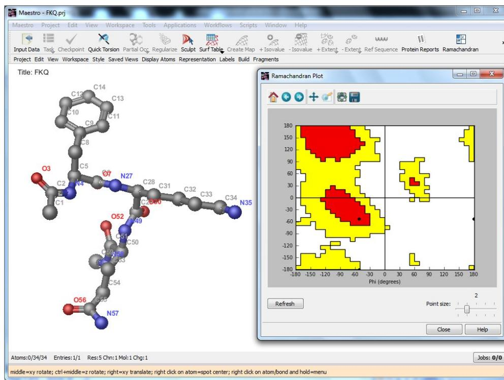
Figure 8. Ramachandran plot representation of tripeptide *Phe-Lys-Gln* (FKQ) in the four Quadrant Square with its chemical inbuilt showing Carbon, Oxygen and Nitrogen atoms at respective positions.
