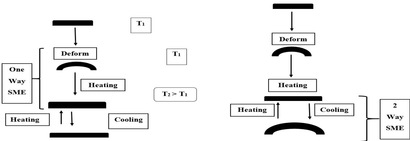
**Fig. 3:** One way and two way shape memory effect.
