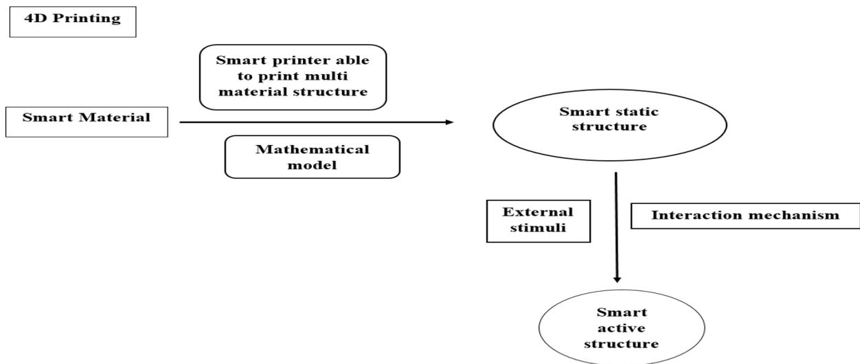
Fig. 2: Basic mechanism of 4D printing.
