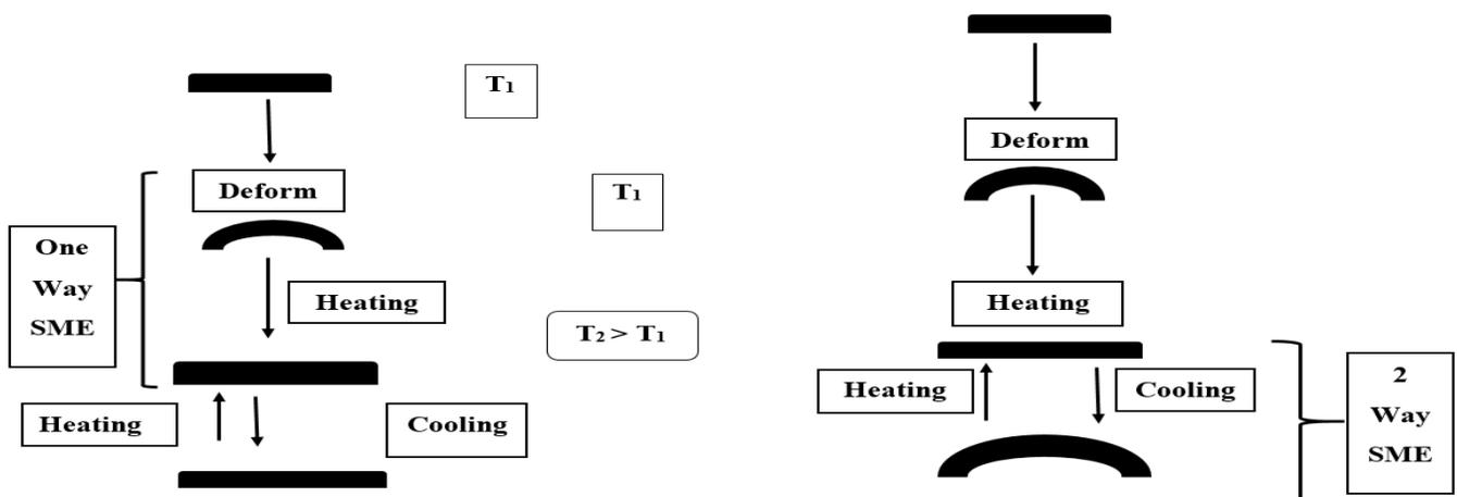
Fig. 3: One way and two way shape memory effect.
