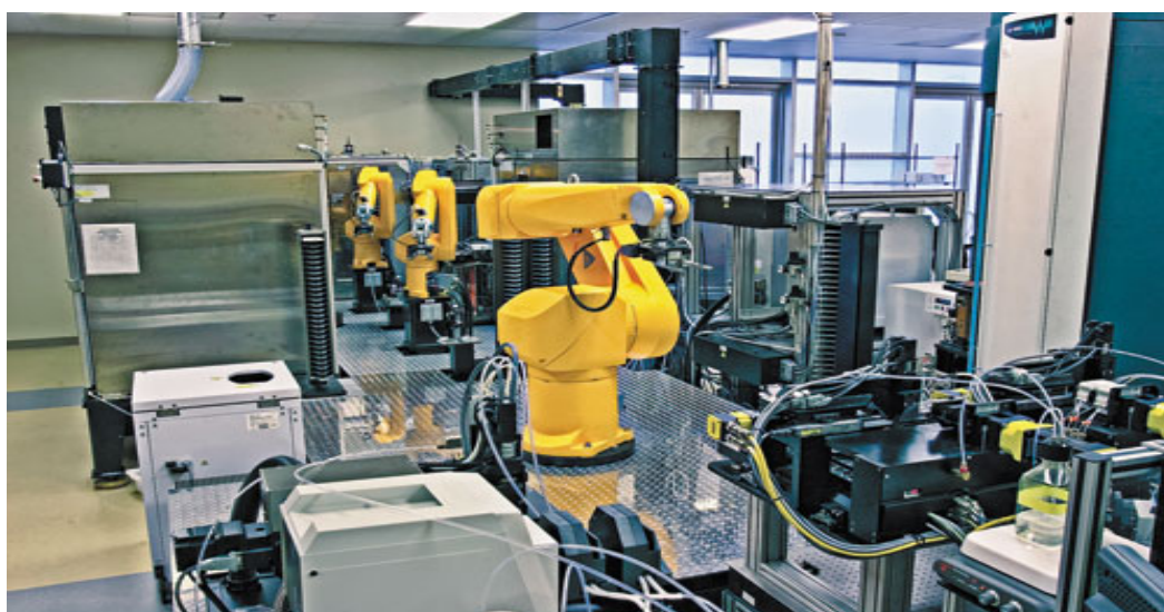
Fig.: High-Throughput Screening Robotics
