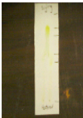
Fig. 3. TLC profile of the methanol extract of H. schizopetalus leaf. Solvent system: ethyl acetate: methanol (7: 3). R_f values: 0.44, 0.53, 0.74, 0.82.
