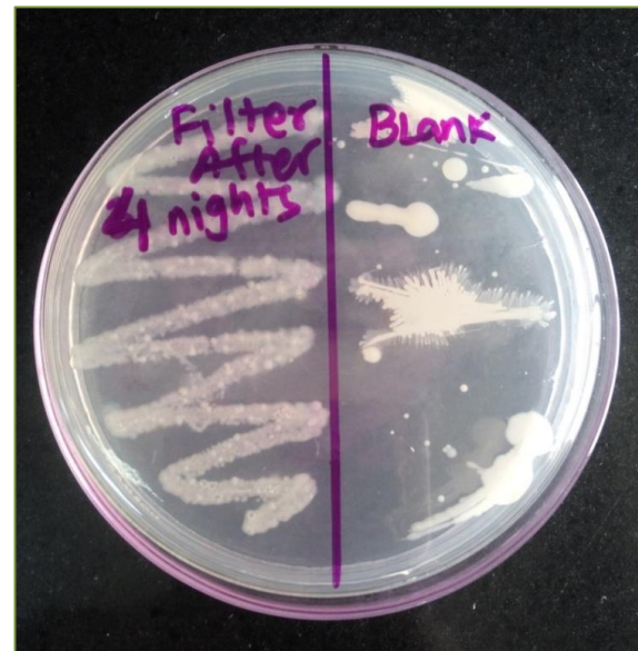
Figure 7: Growth of bacteria in water treated with charcoal and left for 4 nights observed in the agar plate
